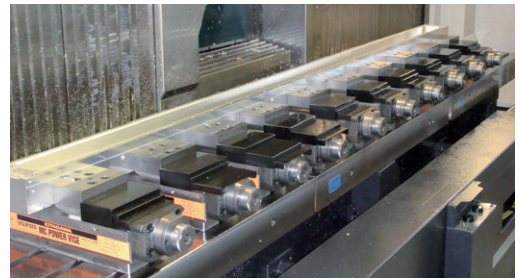
▲3mリアテーブルのM/Cにバイス10台を並列仕様で搭載 ▲On the 3 m linear table, 10 vises are mounted with the parallel specification.
