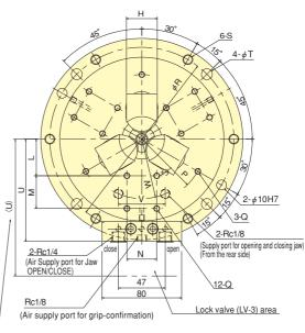
\*By opening jaws the chuck clamps ID of the workpiece.
