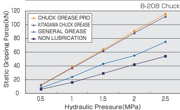
**Fig.2 Grease Check Test**
